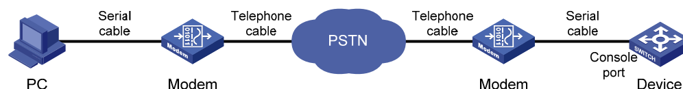
Figure 19 Set up a configuration terminal
