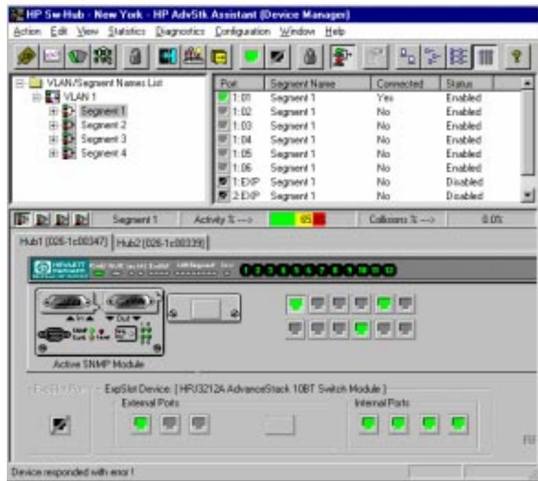
Figure 11-1. Switching Hub Closeup View
