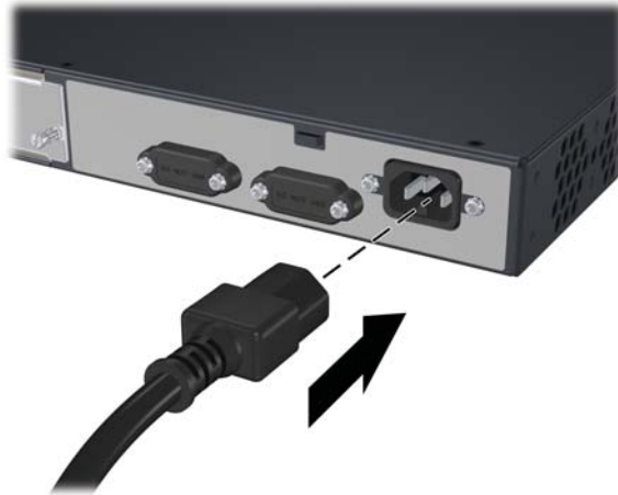
Figure 2-5. Connecting the power cord.
