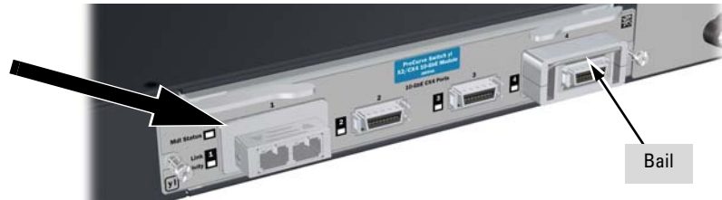
Figure 2-3. Securing a transceiver bail.
