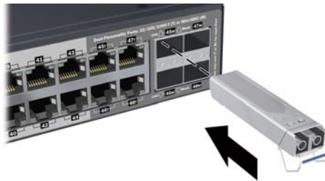
Figure 2-4. Installing a mini-GBIC.
