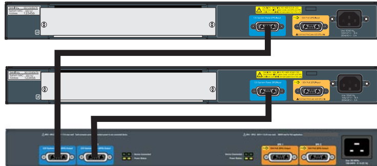
Figure 2-13. Connecting RPS to 2, 24 port switches.
