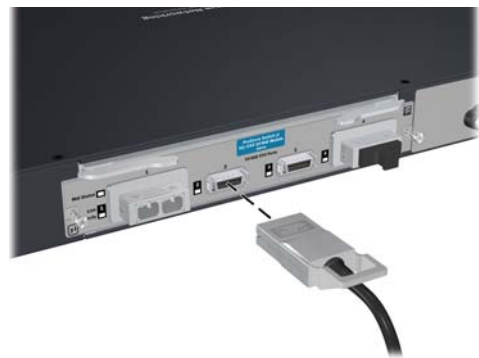
Figure 2-11. Connecting copper cable.
