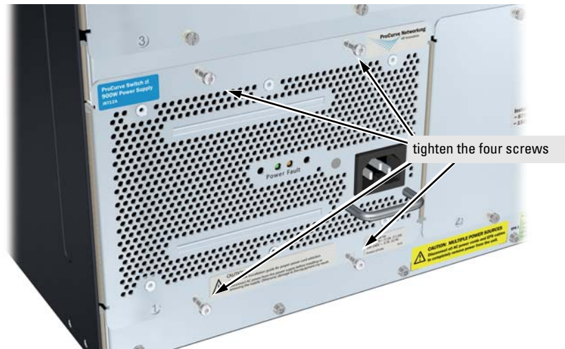
Figure 2-8. Back of Switch with Power Supply Fully Installed
