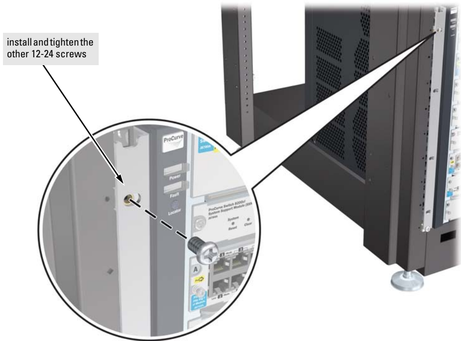
Figure 2-5. Screws in Bracket Being Installed
