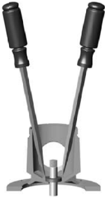
Figure 13 - Remove Mechanical Seal
