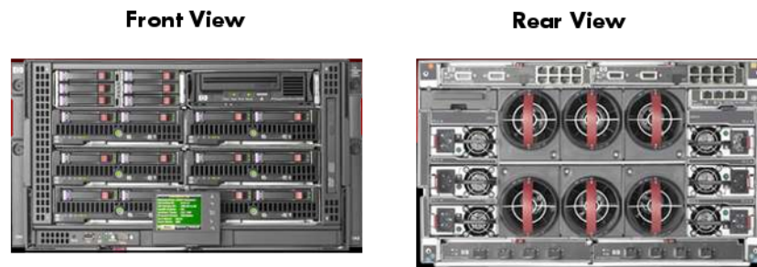
Figure 1-5 HP BladeSystem c3000 Enclosure (Front and Rear Views)
