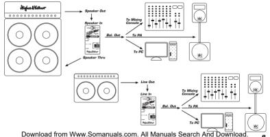
The Hughes & Kettner Red Box Classic converts Line Out and Speaker Out signals into balanced, frequency-compensated signals, enabling a direct feed to a mixer. The Red Box Classic features two voicing options, a 4x12° cabinet and a 2x12° combo.
