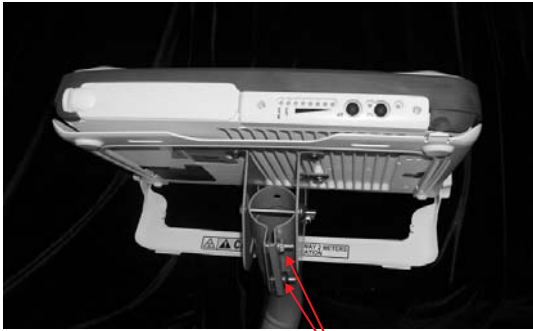
Loosen these fasteners to adjust azimuth
