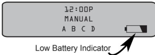
When the Low Battery Indicator appears it is best to change the batteries at your earliest convenience. Install two fresh AA Batteries.
