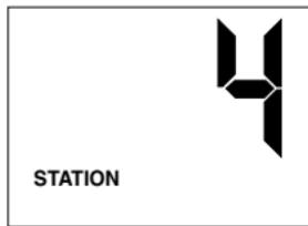
The ICR system will allow you to remotely turn on and off any station on your Hunter controller with the press of a button. Once on, the station will run for the run time you have designated in the ICR transmitter.
