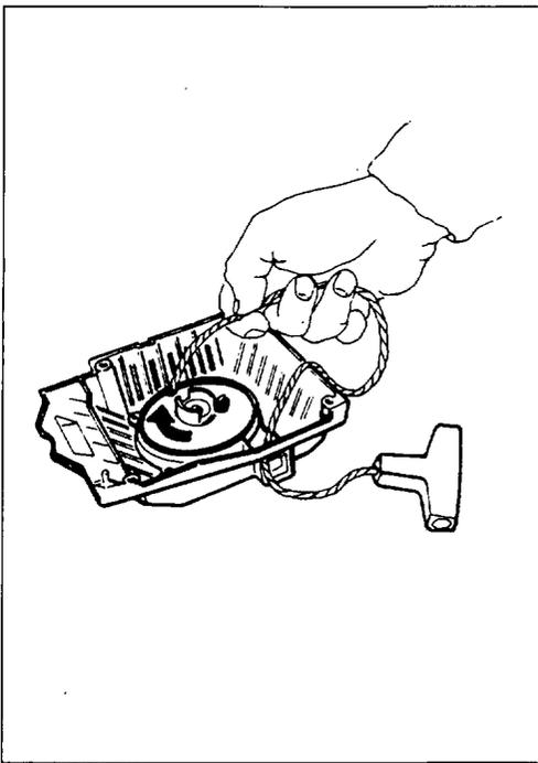
**(Eng) Tensioning the recoil spring**
